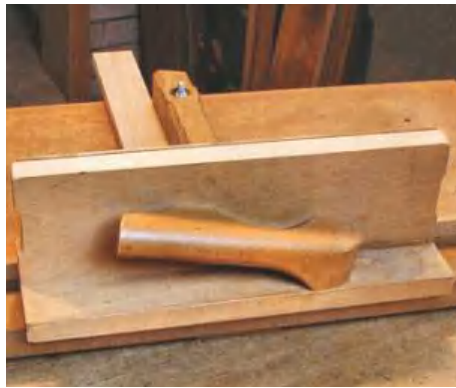
▲ Pic.5 ...such as the ergonomically shaped handle, or tote, on the sanding jig
